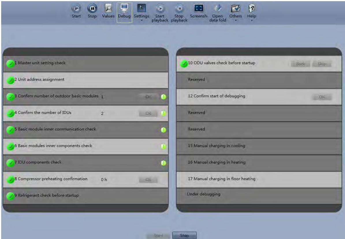
In step "11 Select charging method", the system automatically selects manual or auto charging mode. You can directly choose manual charging. If no operation is performed within 3 minutes, manual charging is automatically entered.
