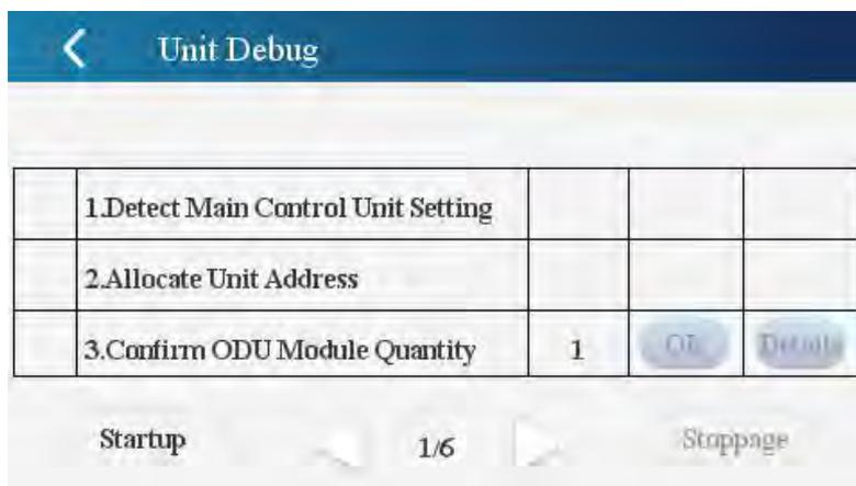
**Step 6:** During commissioning, multi-functional debugger shows the current process (step). In steps 3, 4, 8, and 12, click Confirm to go to the next step. In step 10, click Skip or Back. In steps 3, 4, 5, 6, and 7, you can view the details.
