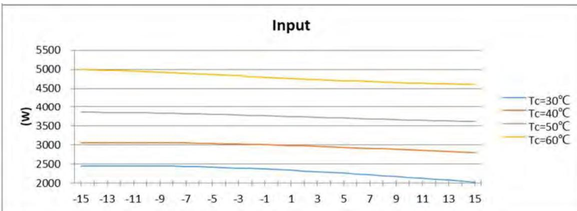
When the compressor frequency is 60 Hz, the power curve corresponding to the evaporation temperature and condensation temperature is shown as follows:
