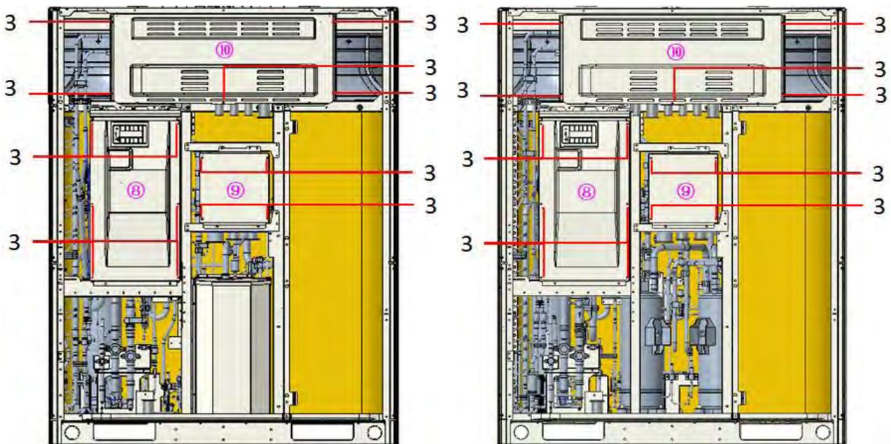
3—screw      ⑧—lower electric box cover      ⑨—upper electric box cover      ⑩—middle electric box cover
