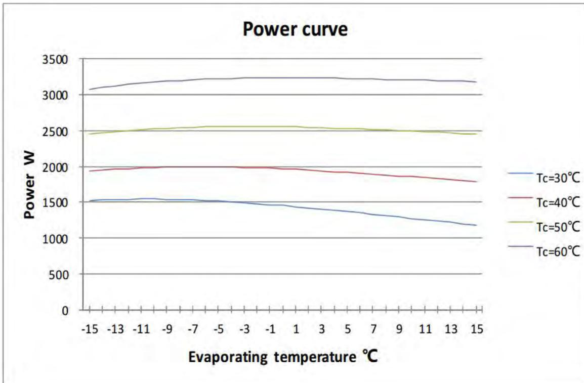
When the compressor frequency is 60 Hz, the power curve corresponding to the evaporation temperature and condensation temperature is shown as follows:
