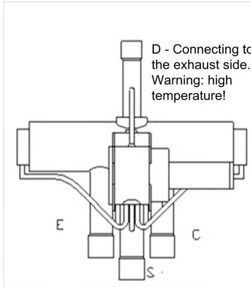
There are labels in the 4-way valve, D refers to connecting exhaust side, S refers to connecting inhalation side of gas-liquid separator. When the system is operating, check if the temperature of the pipelines are the same with that of the following table. Note that do not directly touch the pipeline for avoiding scald!
