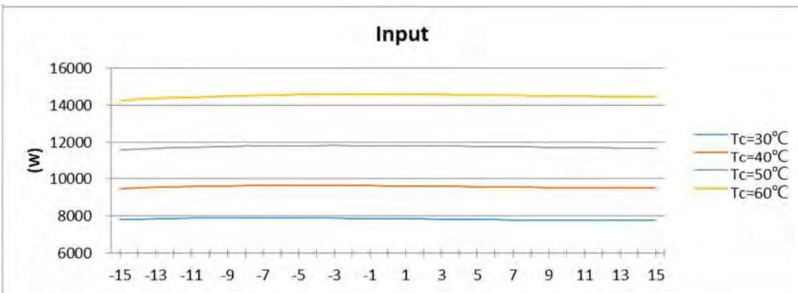
When the compressor frequency is 120 Hz, the power curve corresponding to the evaporation temperature and condensation temperature is shown as follows:
