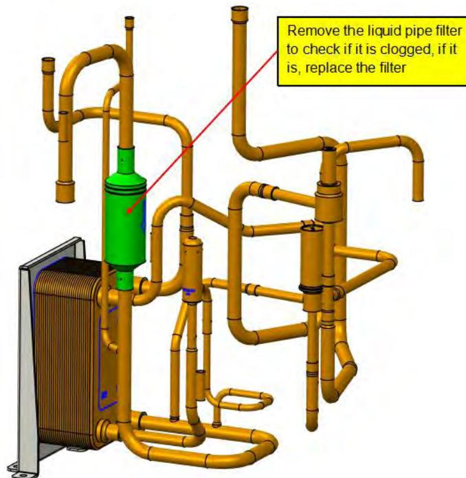
Remove the other piping components according to the actual conditions. If the components are not replaced immediately after removing the pipeline, use tape to seal the pipeline to prevent moisture and impurities from contaminating the system.
