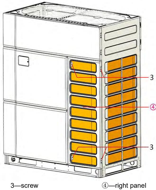
5.1.1.1.4 Remove the unit cover plate (front), panel component (double fans), left panel (lower) (GMV-Q96/120/144/168WM/C-F(U)、GMV-VQ72/96/120WM/C-F(U))
