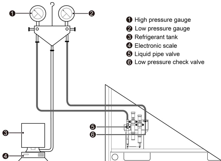
**Step 2:** Fully open the liquid pipe valve and gas pipe valve of each module.
