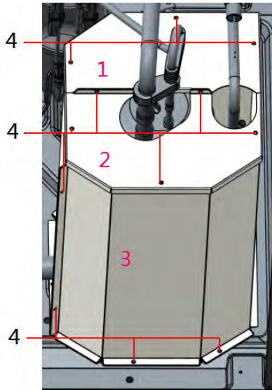
1—upper cover plate 3    2—upper cover plate 4    3—side plate 3    4—screw
