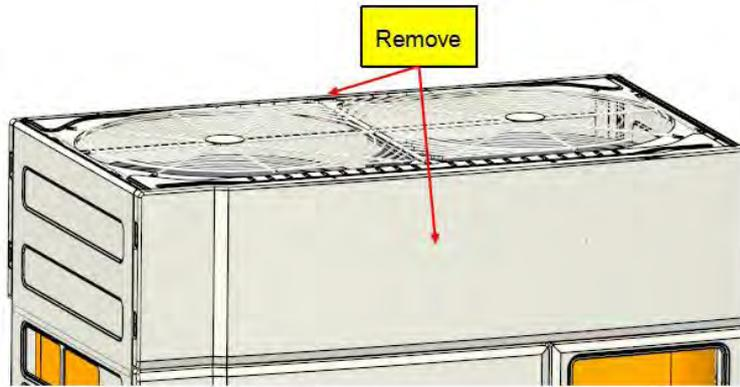
②. Remove the fixing screws.
