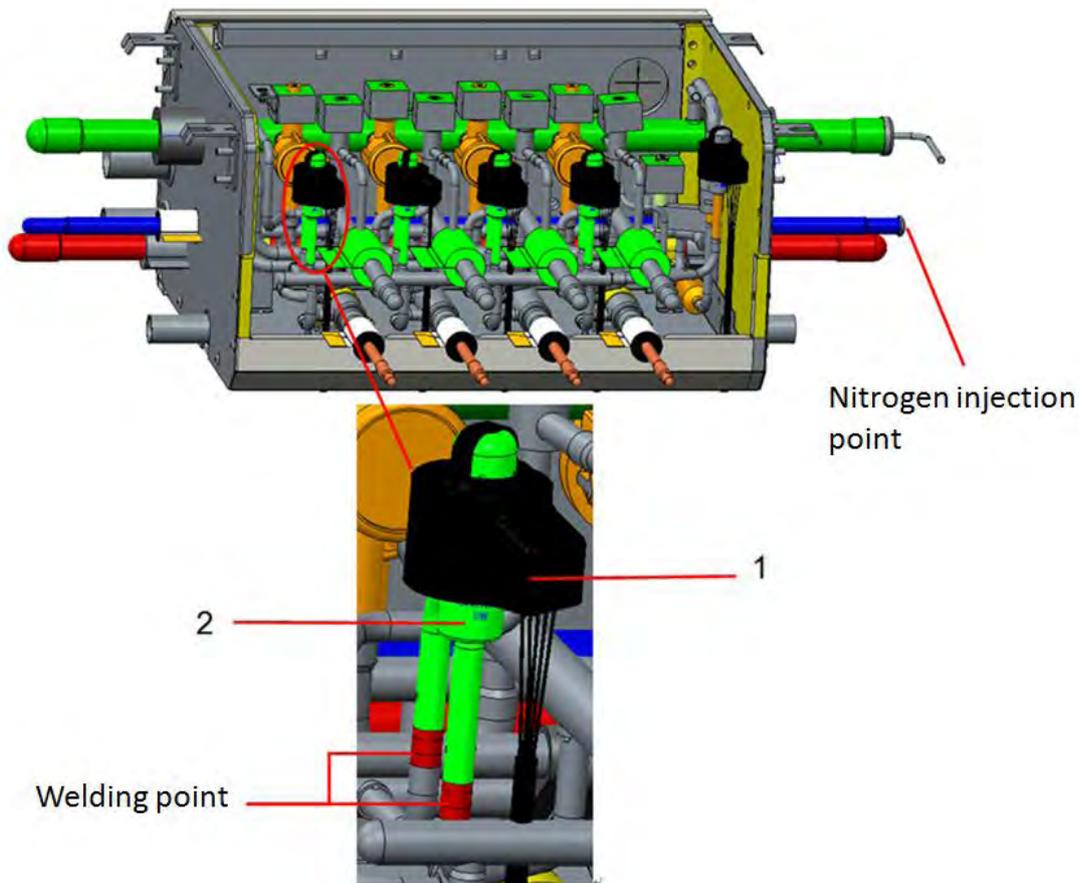
1- electronic expansion valve coil
