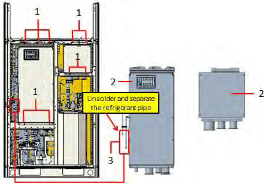
② Before removing, loosen the two refrigerant tubes of the electrical box radiator.
