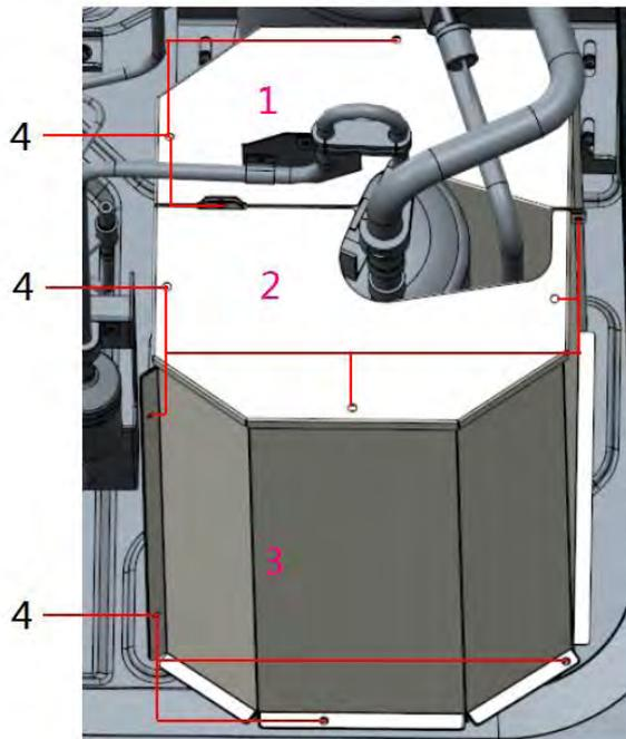
1—upper cover plate 1    2—upper cover plate 2    3- side plate 3    4—screw
