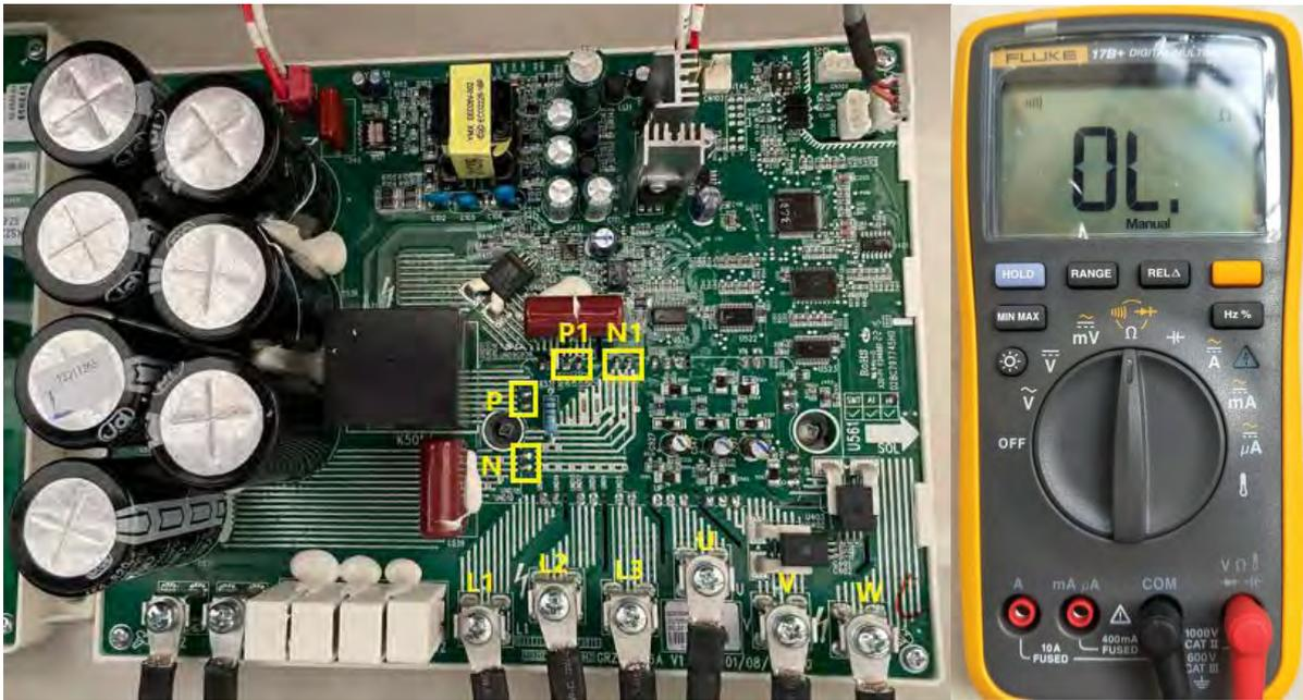
**3:** Point the black probe to the P bonding pad and the red probe to the L2 wiring terminal. In the normal condition, the multimeter will not beep. If it does, the drive board is damaged and needs to be replaced.
