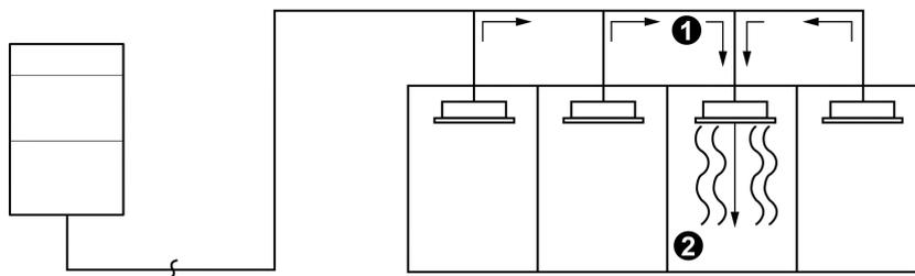
❶ Flow direction of refrigerant leakage
