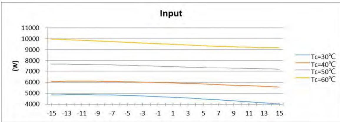
When the compressor frequency is 90 Hz, the power curve corresponding to the evaporation temperature and condensation temperature is shown as follows:
