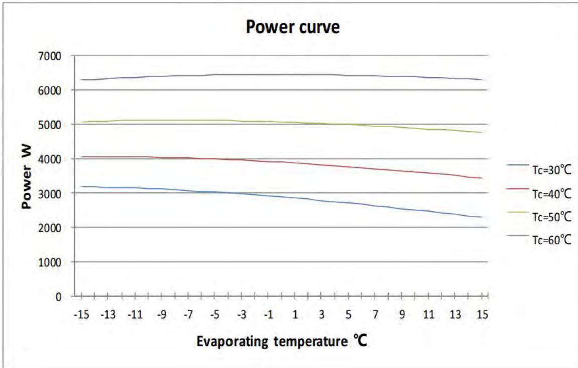
When the compressor frequency is 90 Hz, the power curve corresponding to the evaporation temperature and condensation temperature is shown as follows:
