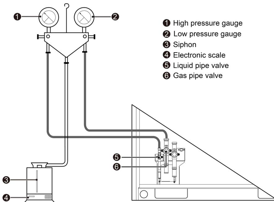
**Step 5:** Open the high pressure gauge valve (the low pressure gauge valve remains closed), charge the system with refrigerant, and record the weight change of the refrigerant tank.
