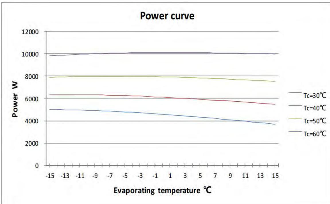
When the compressor frequency is 120 Hz, the power curve corresponding to the evaporation temperature and condensation temperature is shown as follows:
