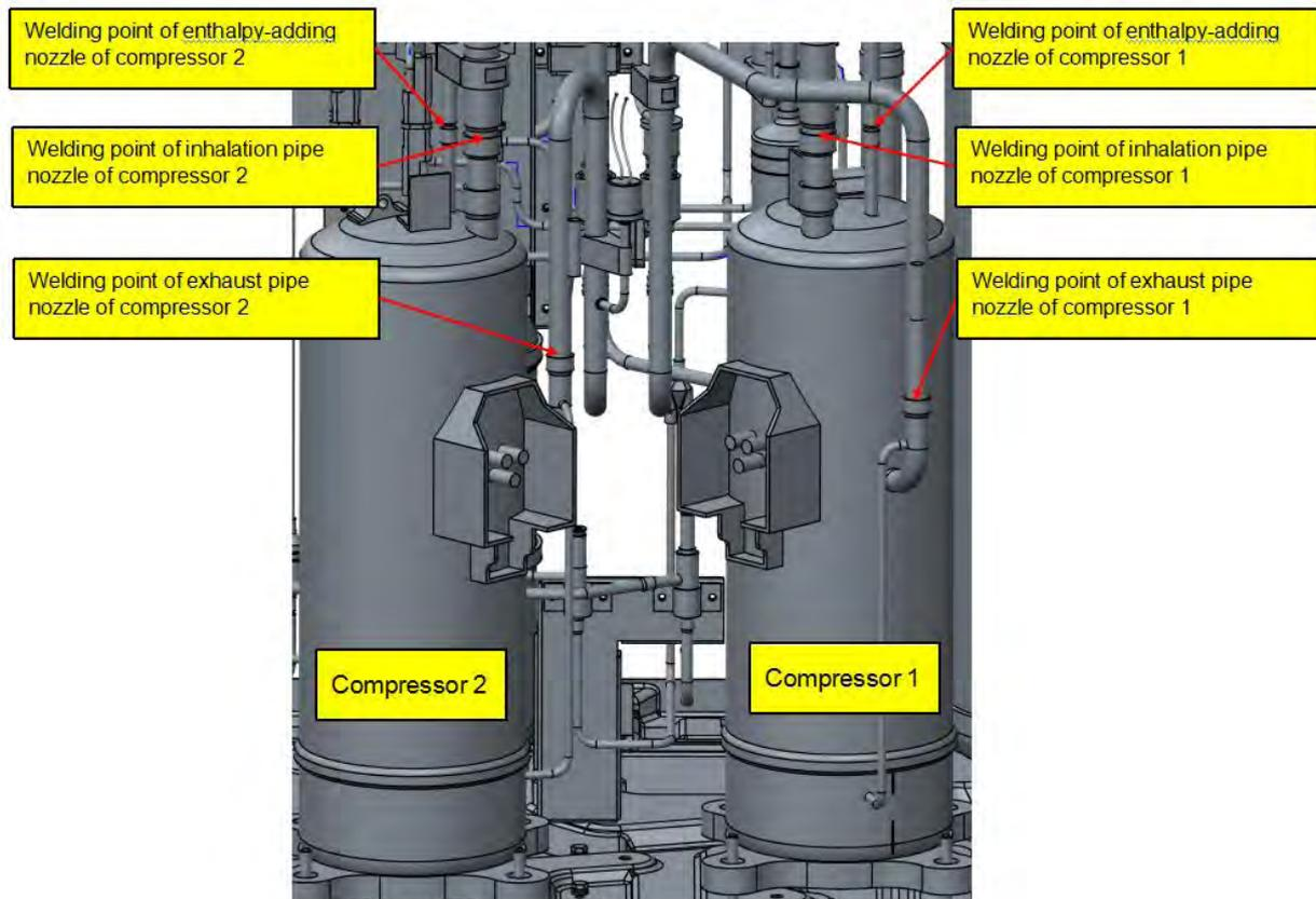
Before replacing the compressors, make sure that the models of the compressors to be replaced are same as the models of the new compressors. The new compressors must be installed at the same places of the respective old compressors and wired correctly. We recommend you replace the compressors one by one.
