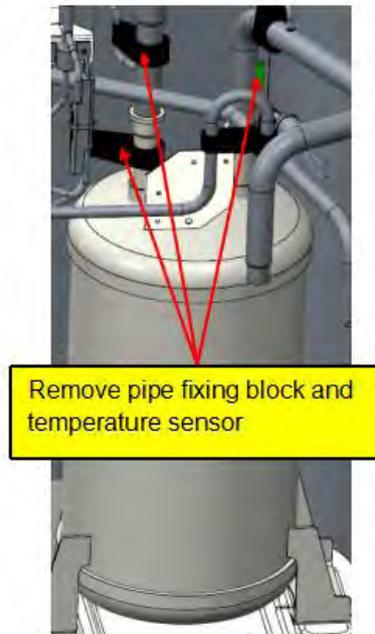
(3) Remove the fixing bolt, take away the gas-liquid separator.
