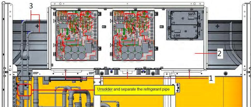
1 — screw 2 — electrical appliance box 3 — radiator refrigerant tube
