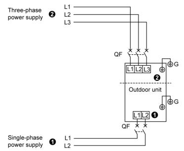
NOTE: For single-phase units, connect wires according to drawing (1); for three-phase units, connect wires according to drawing (2).
