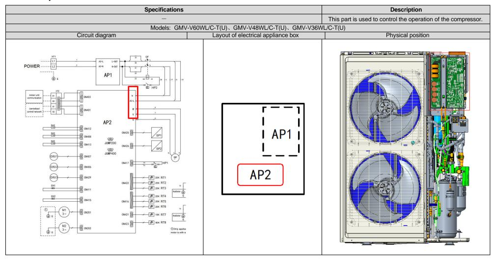
(1) Before the inspection: Find a correct digital multimeter and switch it to the diode gear. Power off the unit and wait two minutes. Disconnect the U, V and W cables of the compressor and N and AC-L power cables from the main board. Do not operate without waiting two minutes after the unit is powered off.
